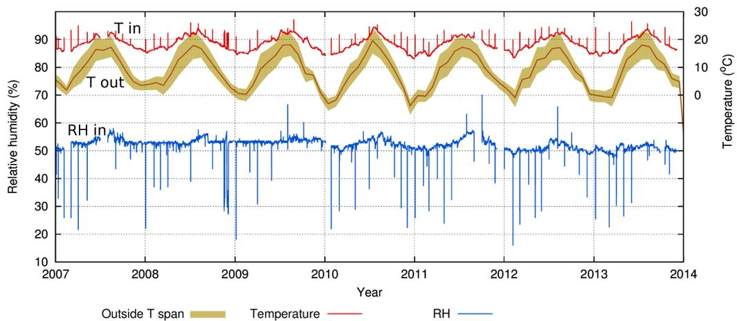
Figure 4: A record of the archive climate over seven years, compared with the monthly average outside temperature and temperature span. The spikes show the climate in the conservator’s office when the logger was retrieved to extract its data.
