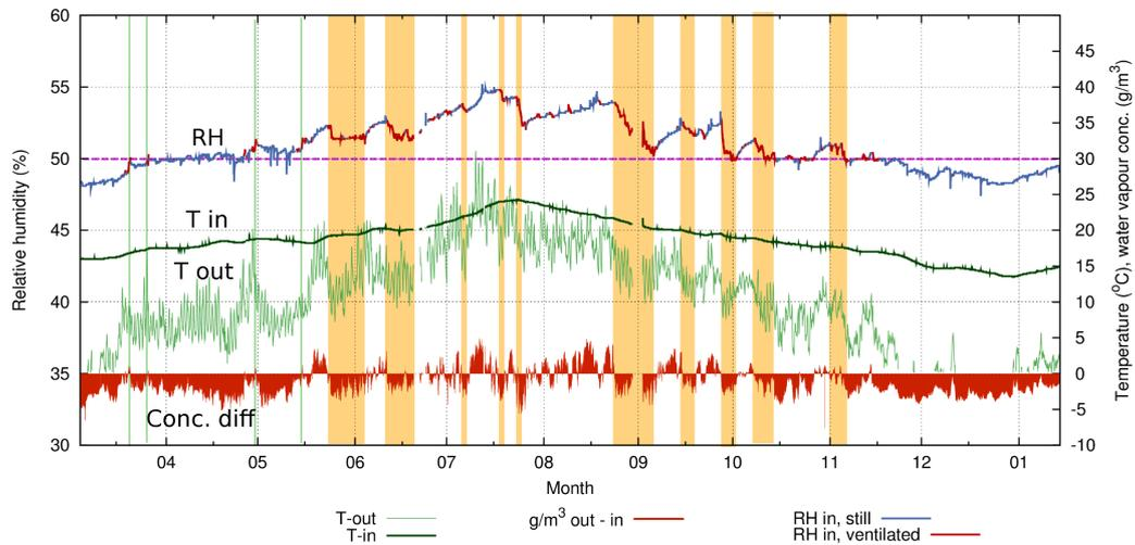
Figure 5: The year 2010 in the archive. The shaded vertical strips indicate periods when outside air was pumped in to raise the air exchange rate from 0.1 per hour to 0.5 per hour. The shaded strips correlate with the difference in water vapour content between the outside and the archive air. The dashed horizontal line marks the target RH.
