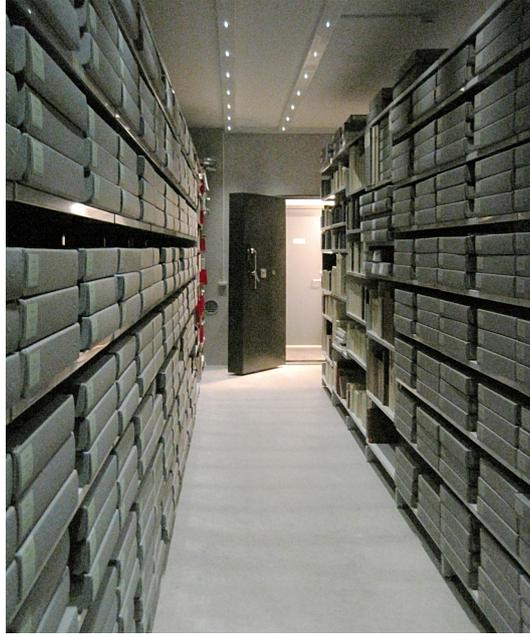
Figure 1: A view of the interior of the archive. It measures  $10 \times 4 \times 3$  m high. The lobby is visible beyond the armoured and insulated door. The duct for pumped outside air is just visible above and to the left of the door.
