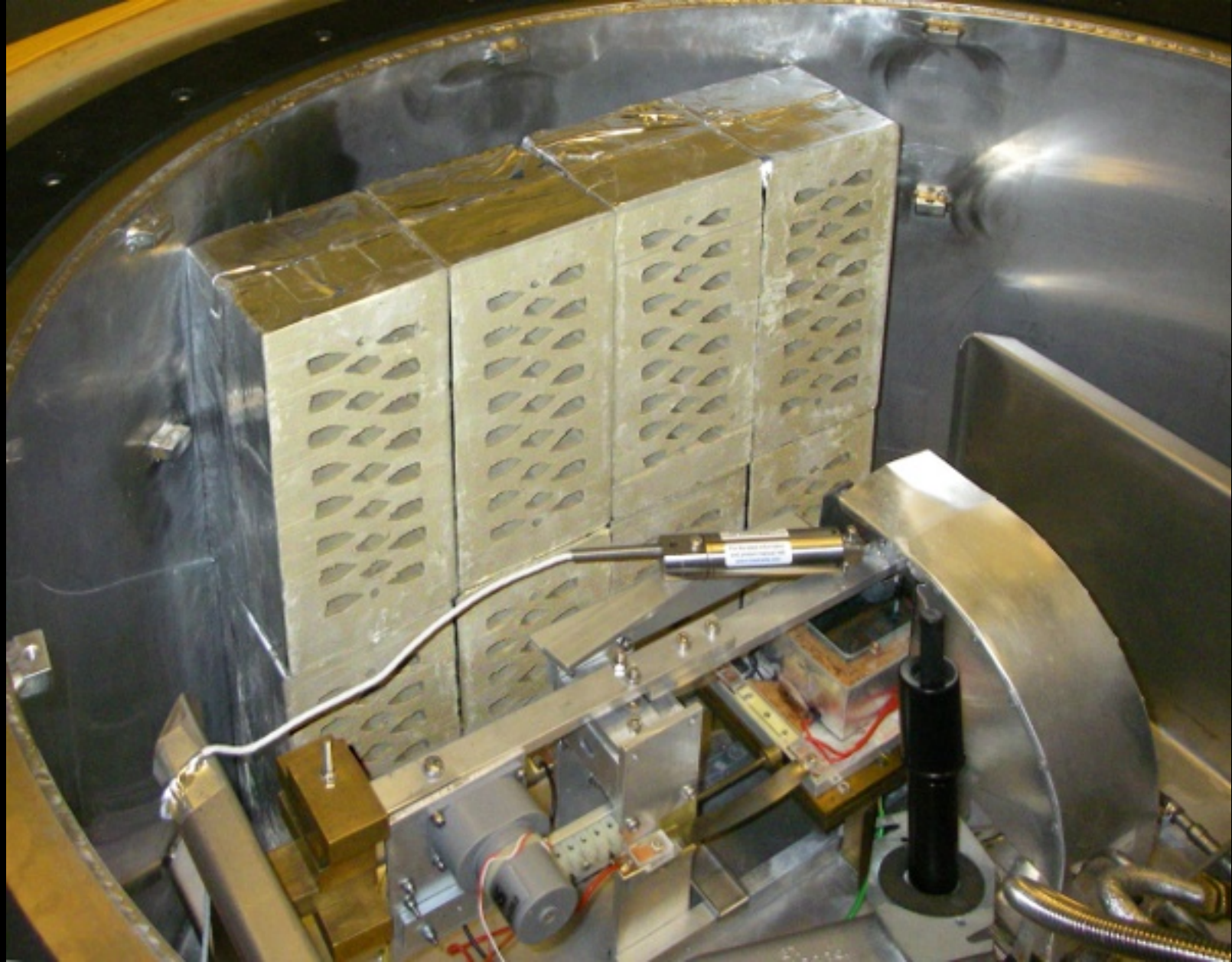
The experimental apparatus. Unfired perforated brick is exposed in an airtight chamber to a fluctuating RH
