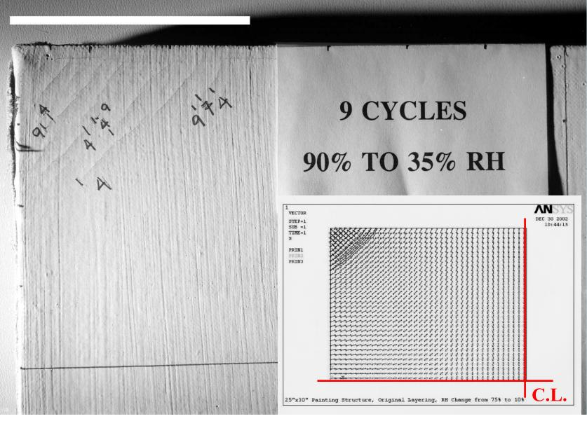
naggainm Buckling from loose keys and over expansion Cracking from low RH Key out cracking
