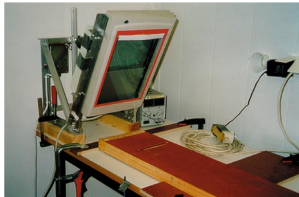
Figure 2. The picture shows the set-up of the climate room with the test piece lying on the workbench. The measurement scale can be seen as a light stripe in the upper part of the plank. The scanner has been moved to the side of the test piece. Photo: Tom-Nils Nilsen
