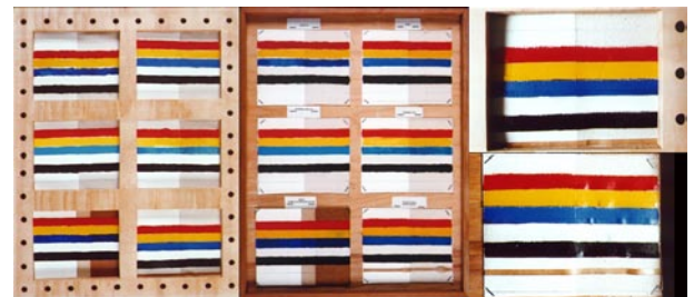
Figure 5. painting replicas exhibited with (left) and without (center) the protection of the glass at the MAC-USP, and details (right) of the mixed media - acrylic, oil and Kraft paper on canvas samples, protected by the glass box (above) and unprotected (below), showing the paper undulations.
