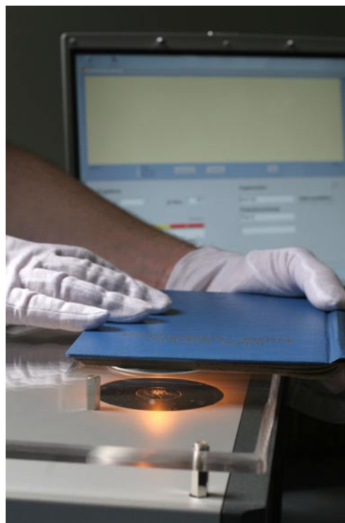
Figure 2. The SurveNIR instrument for non-destructive evaluation of paper chemical and mechanical properties based on chemometric evaluation of NIR spectra.
