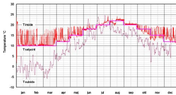
Figure 13. Climate records from Ollerup church, located on Fyn. The temperature is adjusted stepwise to a new set point for each month. The church is heated to 18°C for services.
