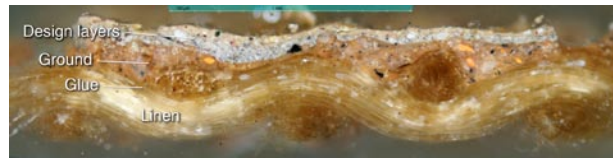
Figure 4. The construction of a traditional canvas supported painting. This assembly includes the “support” canvas, a glue size layer, an oil ground and the oil design layers. This particular section was from a 19th century Italian painting. The green bar at the top of the picture is 1mm. (The cross-section and photograph courtesy of Melvin J. Wachowiak)
