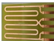
and after 141 days of testing. A slight corrosion is visible at the left lower part of the copper layer.
