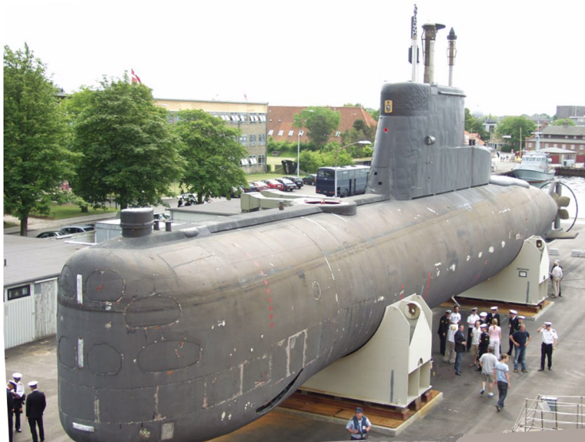
Figure 3: A submarine at the Copenhagen waterfront, which is now transformed into a museum and open to the public. The inside temperature is very unstable due to heat gain and loss by radiation.
