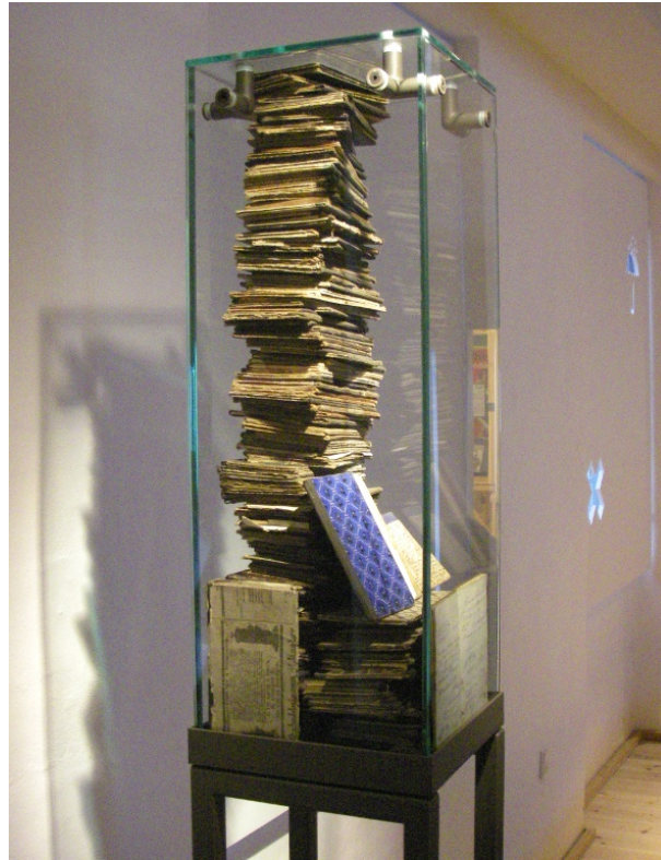
Figure 11: A display case at the Museum of Industrial History in Brede. The paper content will buffer the RH inside the case over the whole year if the leakage rate is low.
