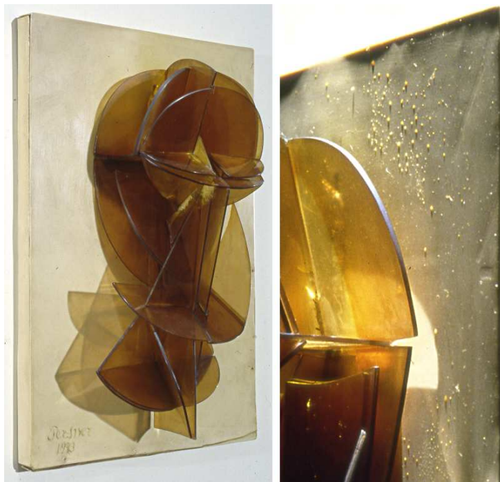
FIGURE 16. Head of a Man, by Antoine Pevsner, in the collection of the Hirshhorn Museum, Washington D.C. The raking light picture on the right shows droplets of calcium nitrate solution. This is the product of the reaction between nitrogen oxides released from the decomposing cellulose nitrate with the calcium carbonate (chalk) filler in the white celluloid back plate. Calcium nitrate is deliquescent, so the water component comes from the air.
