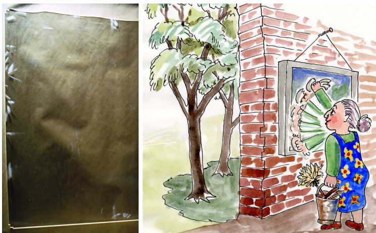
FIGURE 21. Not all contamination in enclosed spaces is caused by diffusion and convection. This acrylic glazing (left, about 1m square) protected a confederate flag in the Battle-field Museum at Fredricksburg, Virginia. The strange feathery deposits along the edge are gypsum. The source is the wall behind the picture. The gypsum moved in solution in water penetrating the outer wall and migrated into the board supporting the flag. It would have stayed there, but for the enthusiasm of the cleaner, whose cloth generated an enormous electrostatic field where the acrylic glazing met the metal frame (we have reproduced this process in the laboratory).
