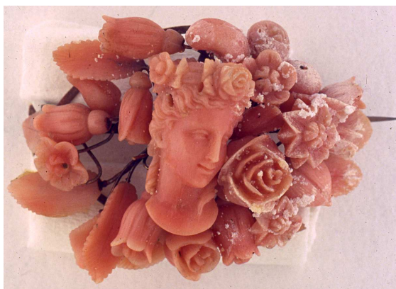
FIGURE 2. A coral brooch, 4cm long, which had been stored for many years in an oak barrel, together with other ornaments made of cellulose nitrate. The white corrosion is cellulose acetate-nitrate.
