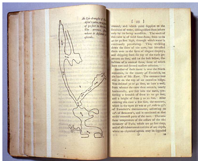
FIGURE 15. This book had only been exhibited for a few weeks in a temporary exhibition before the strong yellowing of the paper was revealed by the paler paper preserved under transparent polyester strips which restrained the pages. The damage cannot have been caused by light but must be due to chemicals in the air. The reactivity of the gas is emphasised by the greater yellowing immediately adjacent to the strips and at the edges of the pages. A pollutant absorber discretely placed in a remote part of the case would not have given protection.
