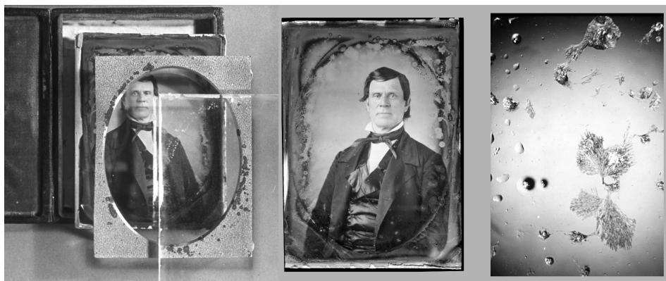
FIGURE 9. A Daguerreotype, disassembled to show the typical method of presenting and protecting the delicate silver image. The centre of the image is protected by the edge of the silver plate which absorbs hydrogen sulfide diffusing past the edge of the glass. In this example, from the Museum of American History in Washington D.C., the interior surface of the glass has become contaminated. The droplets contain sodium, sulphate and formate ions, with crystals of sodium sulphate and sodium formate. The mixture is deliquescent at the 50% RH of the museum environment
