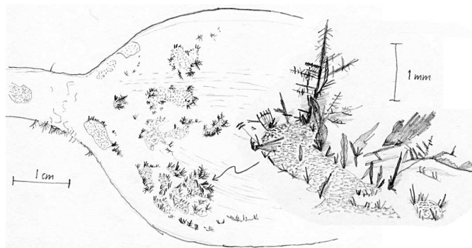
FIGURE 8. A silver spoon from colonial Virginia with a luxuriant furry growth of silver sulfide crystals. To the right is an enlarged detail. Hydrogen sulfide had penetrated cracks in the varnish and attacked the silver chloride layers formed just below the silver surface, by underground corrosion.
