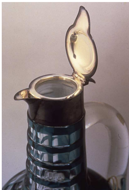
FIGURE 14. The lid of this silver topped decanter provides sacrificial protection of the silver within the neck. Even though the lid is a simple drop fit, the silver reacts so completely with hydrogen sulfide gas that none penetrates to the interior.
