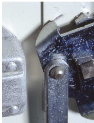
FIGURE 20. The lock of this new storage cabinet corroded on the inside during a few weeks of storage before use. It is likely that the paint had been over-baked in an attempt to remove solvents, generating low molecular weight decomposition products.
