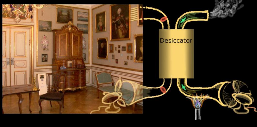
Dehumidification can be achieved by condensation as already explained but it can also be done by sorption into a desiccant which is intermittently regenerated by passing hot air from outside through it. With a rotating desiccant drum the process can be made continuous
