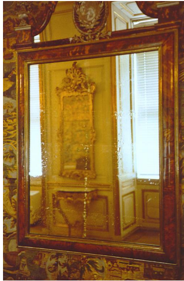
Figure 6: A silver mirror damaged by exposure to -30^{\circ}\text{C} . Physical damage is difficult to see on less optically perfect objects. The record of the appearance of an object before cooling is seldom detailed enough to convince that no change has occurred.
