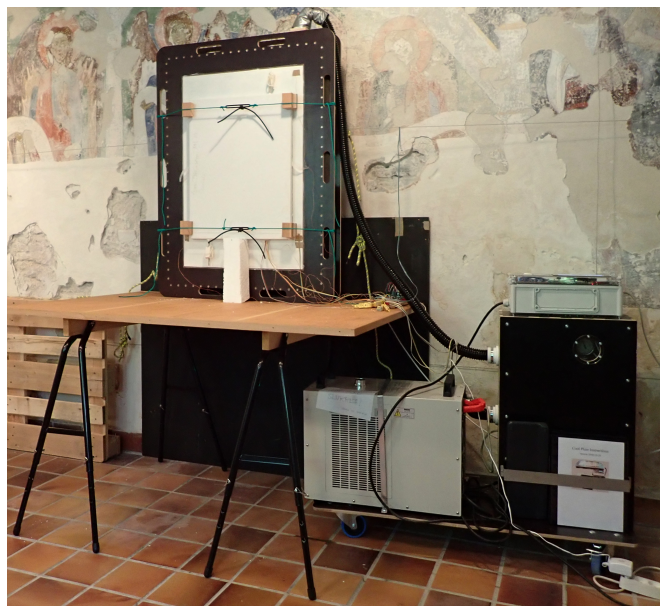
Figure 3: The experimental painting mounted vertically against a “wall” of painted aluminium which is enclosed flush with a plywood frame.
