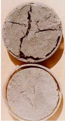
Figure 4.25 The bentonite - perlite mixture shrinks evenly if it is not restrained (bottom). It is therefore suitable for making clay bricks but less suited to cob methods, where the clay is applied in a plastic state. A formulation suitable for plastering walls has yet to be developed.
