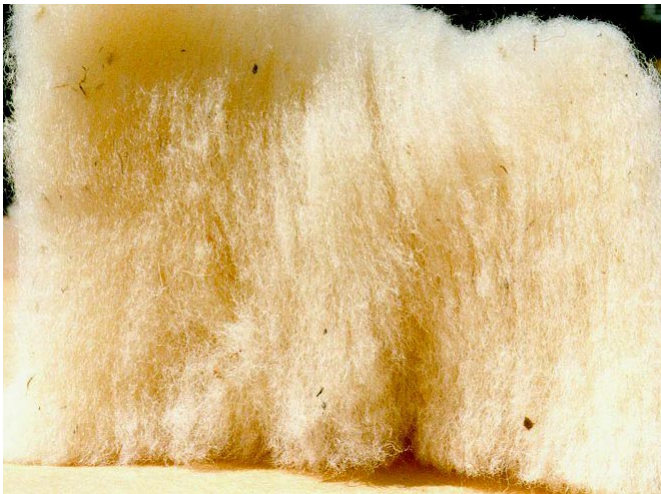
Figure 4.37 Wool insulation. This picture shows a 70 mm section of wool insulation. Notice the laminations parallel to the surface of the slab as it would be installed in a wall.
