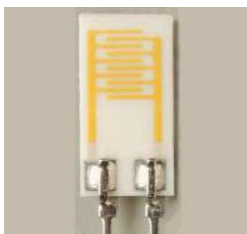
Figure 2.16 The General Eastern RH sensor. It is about 10 mm high. The base is coated with a thin layer of a water absorbent polymer. The resistance between the two gold electrodes is measured.
