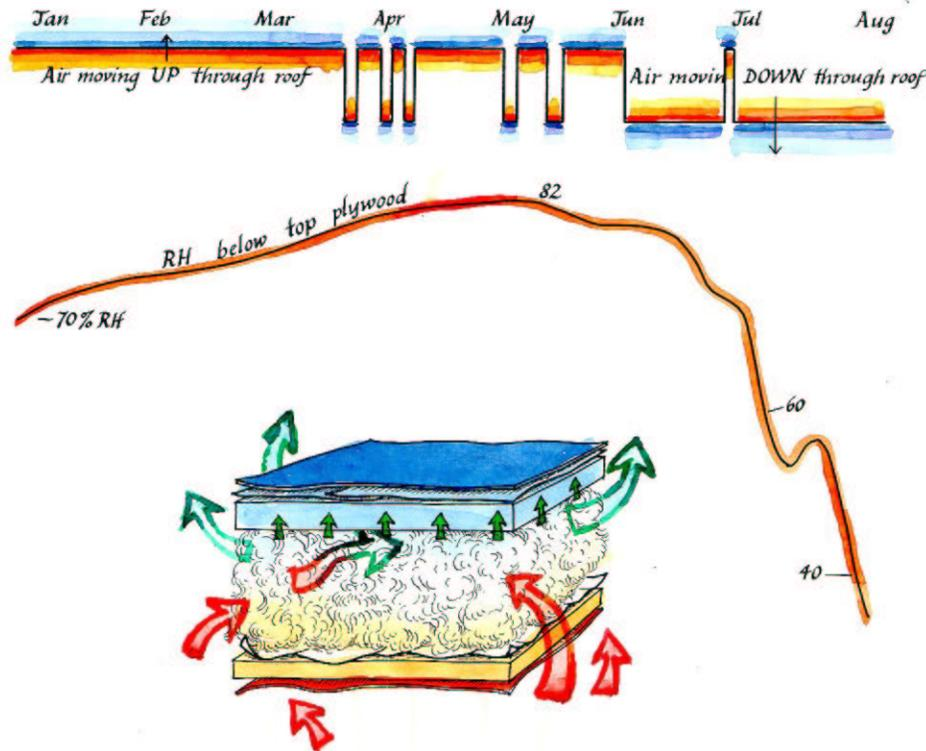
FIGURE 24. Moisture accumulated in the upper plywood layer during the winter, from air flowing between the pre-fabricated roof cassettes. The trace at the top is the direction of air flow through the roof, driven by the stack effect, over a period from winter into summer. Below this is the RH measured just below the upper plywood. Notice the very sharp fall in RH in early summer.
