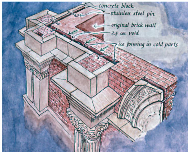
FIGURE 29. During the winter, moist air diffuses from the interior into the gap, which is in many places covered on the outer side with impermeable concrete blocks. The temperature of the gap is uneven, because of the bold sculpting of the facade, so vapour moves laterally to accumulate as ice in the cooler parts.
