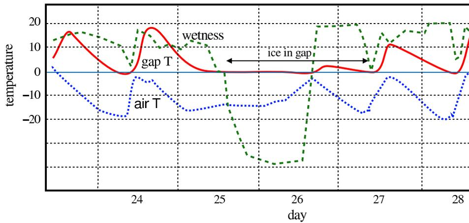
FIGURE 30. A sequence from the climate record showing a period of freezing followed by a long period of thawing, indicating considerable accumulation of ice where the wetness sensor was placed. The wetness sensor measured the surface electrical conductivity of the stone and so gave a 'dry' reading when frozen. Evidence for ice persisting after the wetness sensor has recovered its wetness comes from the slow rise in temperature of the gap at this measuring site
